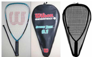
Fig. 1.5 Photo of racquetball bat (a), the bat in a plastic bag (b), and THz wave (0.6 THz) image of the bat in a plastic bag (c)
